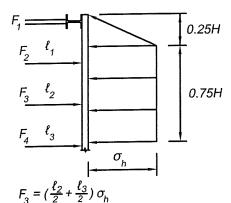
ASSUME HINGES AT STRUT LOCATIONS FOR CALCULATING STRUT FORCES
